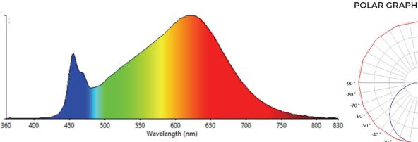
Testing was performed in accordance with LM-79-08.
